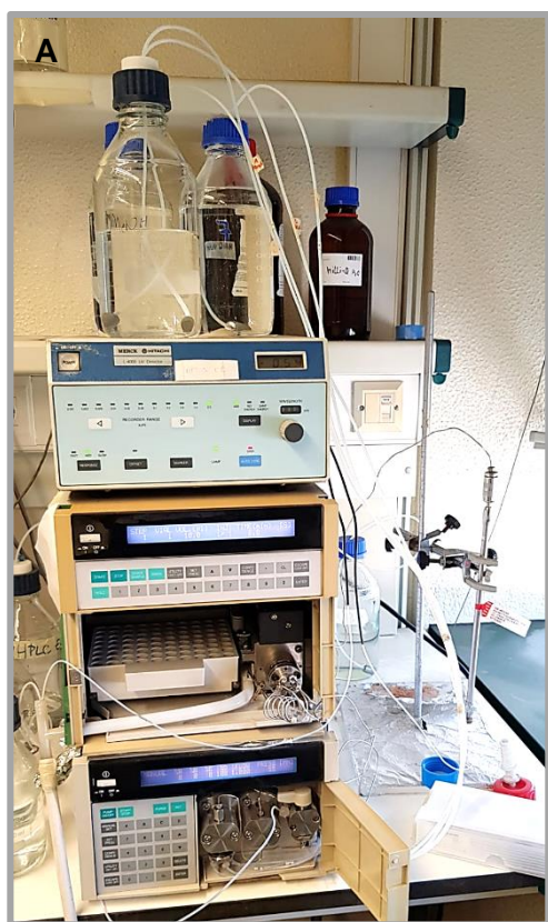
Figure 49. HPLC: (A) Step-up and (B) Chromatogram obtained for artificial mixtures of different proportions between L-DOPA and dopamine: Grey – 75 \mu\text{M} of L-DOPA + 25 \mu\text{M} of dopamine, Pink - 50 \mu\text{M} of L-DOPA + 50 \mu\text{M} of dopamine and Blue – 25 \mu\text{M} of L-DOPA + 75 \mu\text{M} of dopamine. The retention time for L-DOPA and Dopamine, is approximately, 3.13 and 3.45 minutes, respectively.
