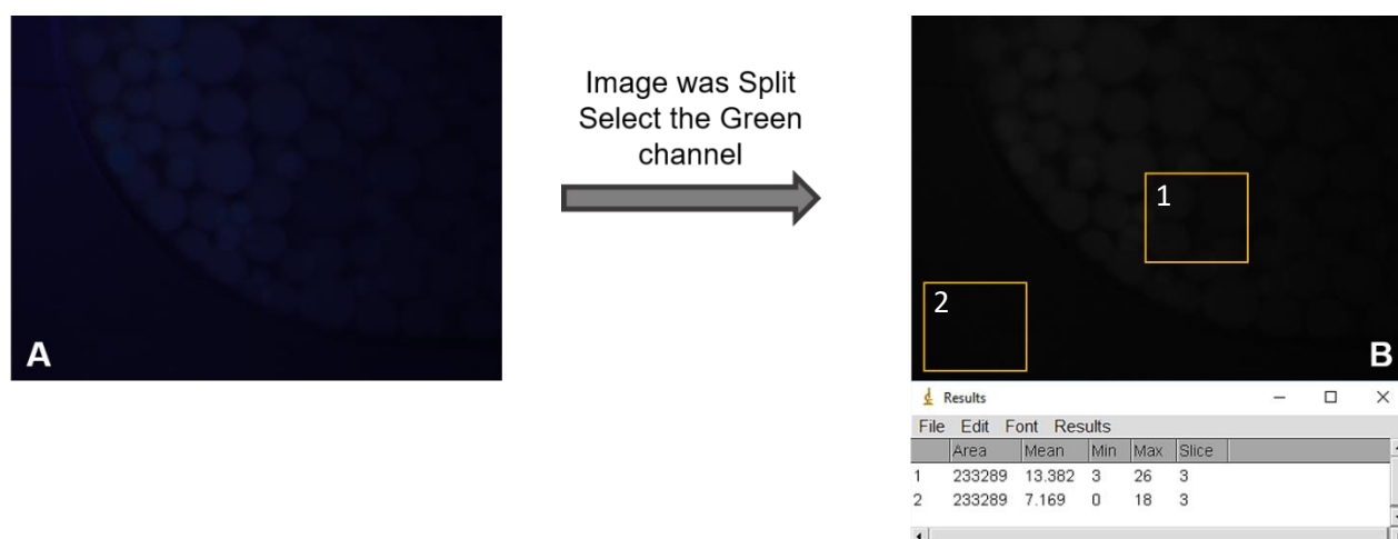
Figure 16. Image Analysis: (A) Source image and (B) Conversion to a green channel, then the value obtained from the outer area is subtracted from the value obtained from the inner area.
